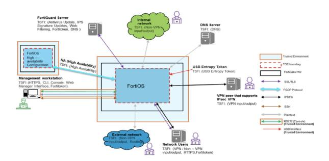
FortiOS (TOE) provides firewall, Virtual Private Network (VPN), Virtual Local Area Network (VLAN), antivirus protection, antispam protection and content filtering to provide network protection for Internet Protocol version 4 (IPv4) and Internet Protocol version 6 (IPv6) networks.
