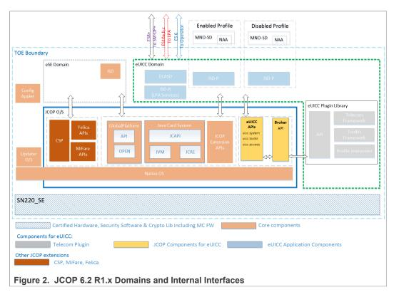
Figure 2 shows the components of the JCOP 6.2 R1.x O/S including the extension APIs for MiFare, Felica, eUICC and CSP. It also shows the Config Applet which has special privileges and is used to personalise and configure the TOE. The eUICC APIs provide access to NXP proprietary functions and a broker API which forwards eSIM/SIM/UICC/ISIM commands to an eUICC plugin library.
