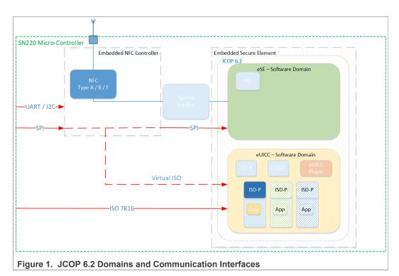
The eSE domain is externally accessible via SPI or by the System mailbox, which is connected to an Integrated NFC controller supporting Type A,B and F contactless communications. The dedicated eUICC Domain is directly accessible by the ISO-7816 interface.
