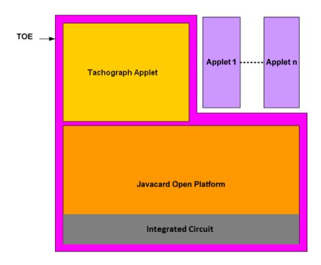
The TOE is composed of 3 subsystems, which correspond to the 3 java packages that form the Tachograph applet (2 applets and 1 library) in the implementation representation. Note that the platform is not covered by the TOE design provided by the developer, although it is considered as an additional subsystem supporting the tachograph applet and implementing some specific SFRs as detailed in the Statement of compatibility of *[ST]*.
