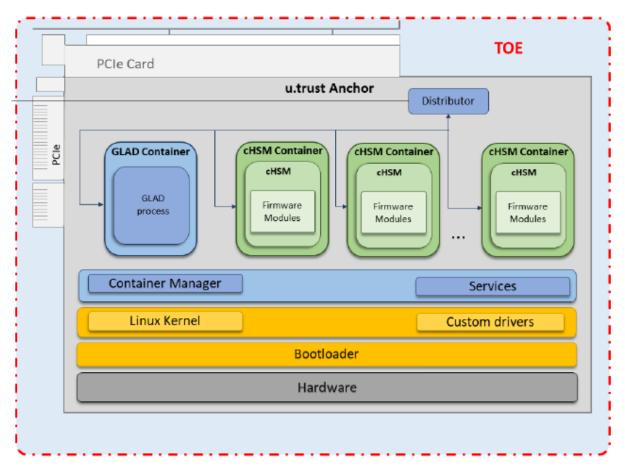
The bespoke Linux kernel is compiled with the minimum features necessary to allow the platform to function, and including security components such as mandatory access control, resource control and other sandboxing techniques.
