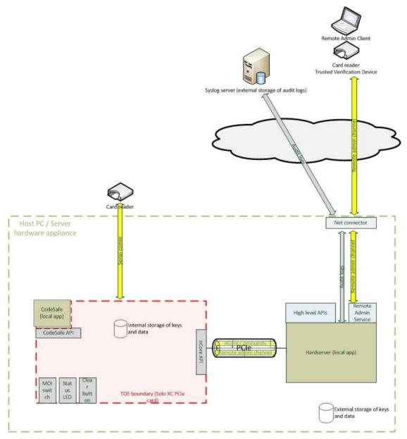
Figure 4 Configuration 2: TOE in host server
