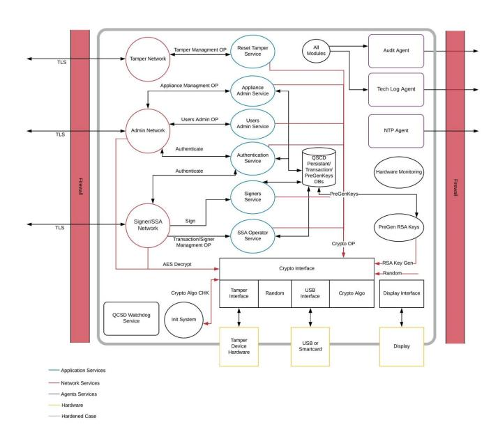
Figure 1. Logical architecture of the TOE
